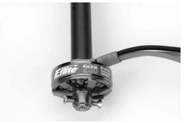
**NOTE:** Photo shows installation using a carbon fiber tube, with 8mm OD, 6mm ID (EFLM1960 available separately). This is an option for mounting the motor. You can cut down the carbon fiber tube to meet your specific needs and attach to your foam or wood airplane with glue.
