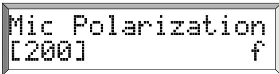
*The flashing (f), the Keyboard Status Indicator, displays which key functions are active. This indicates that the function keys are used for different purpose in current function.*
