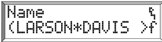
*All but the last of these screens you have seen before. This display is to set one of four custom instrument name screens which will appear each time you turn the instrument on.*
