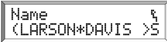
*This one has rounded brackets that mean this is an “entry parameter”. Type the number or character desired (see Chapter 4). If there is an angle bracket “>” then the entry field is too big to fit the screen and will scroll with the
