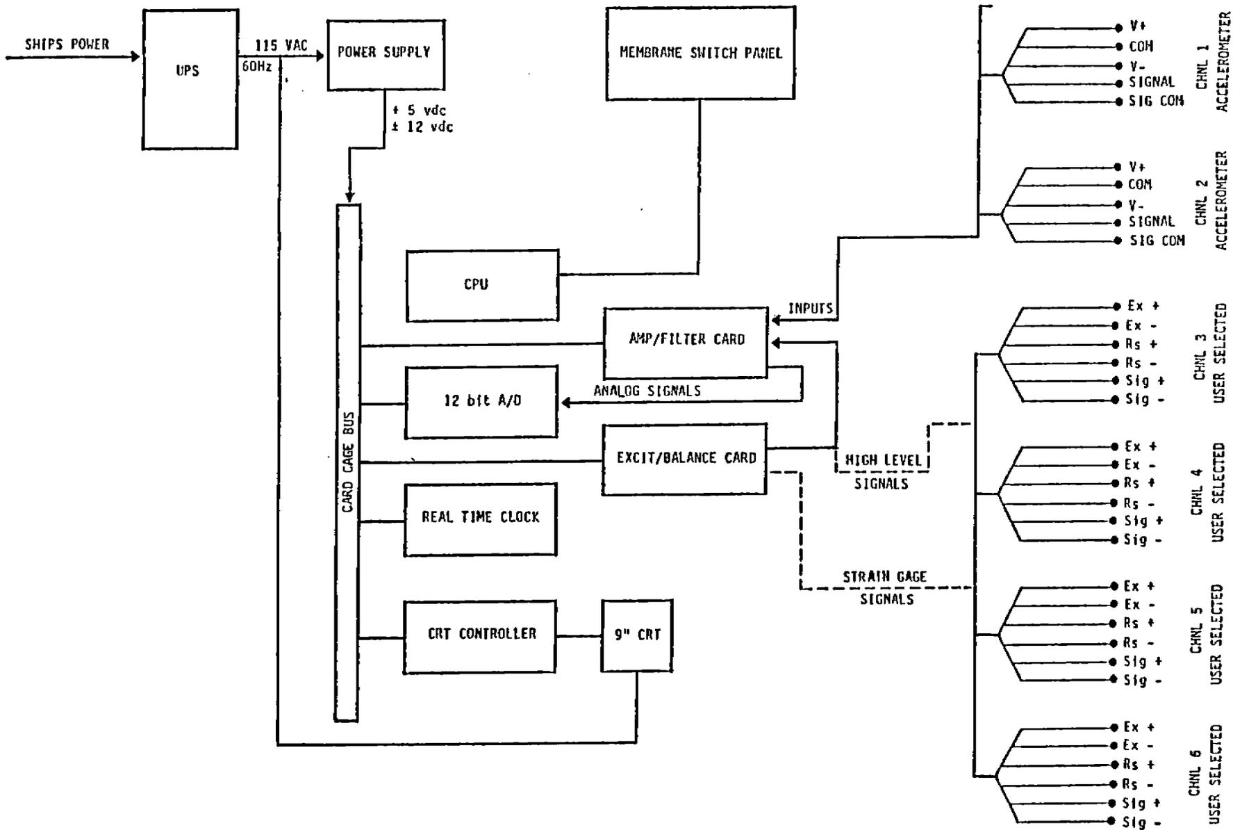
Figure B-3 SYSTEM WIRING DIAGRAM
