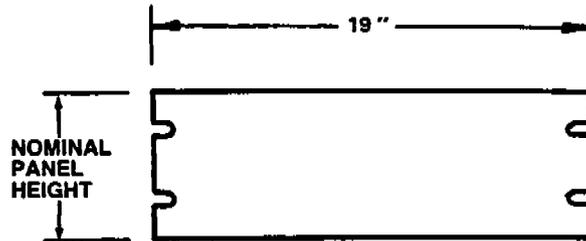
Consoliners may be used as storage, transit or permanent housing for 19" rack equipment with panel heights from 5 1/4" to 26 1/4" high. Like most TA cases, Consoliners are watertight and can be produced to conform to any applicable military specification.
