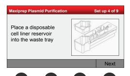
Place the Cell Liner in the reservoir slot in the Waste Tray. Press Next.
