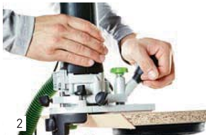
2 Then mill the workpiece flush.
