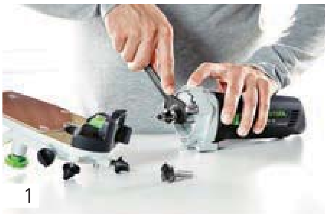
1 First install the router cutter in the MFK 700 Basic.
