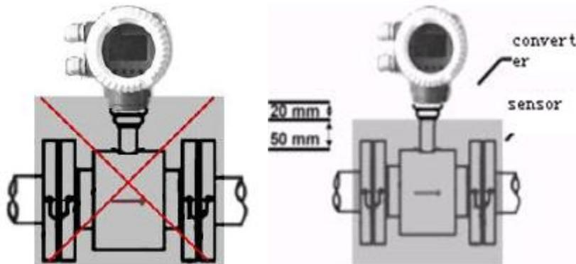
Remark shadow part indicates the right place to cover cotton. If flowmeter has been wrong packed like the left picture shown, the Flowmeter will not work normally due to its heat. The right packet keeps a distance of 20mm between cotton and converter's bottom. Meanwhile, the sensor should be well-packed to prevent the heat.
