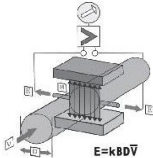
It's measuring principle bases on Faraday electromagnetic induction law :
