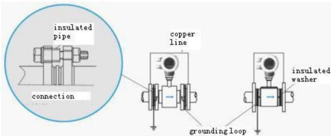
Remark: when sensor installs at the insulated pipe, grounding loop can be avoided.
