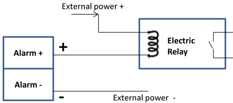
8. Low alarm output wiring diagram (requires external power supply)
