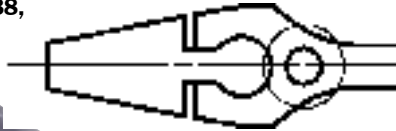
Tapered Jaw For Access Into Tight Spaces.
