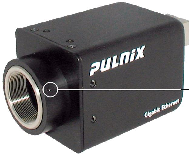
Loosen the three 2mm screws around the perimeter of the C-mount lens collar (two 2mm screws for a CS-mount) to adjust the back focus. Unless you absolutely must, do not attempt to adjust this focus.
