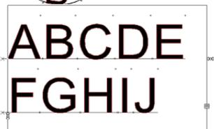
**Horizontal Block Text:** The text is restricted to the width of a block. When the text is wider than the block, it will automatically move to the next line.
