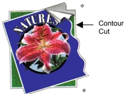
Contour cut is a feature that creates a cutting line around objects, either vector or bitmaps.
