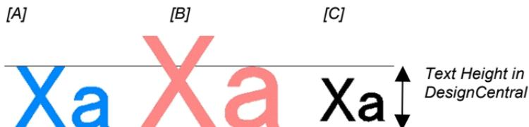
[A] The height of letter “X” was set as a reference in **Based on height of**. The height of letter “X” is exactly the size specified in DesignCentral because it is used as a reference. All other letters, like the “a” in the above example, will be proportionally resized.
