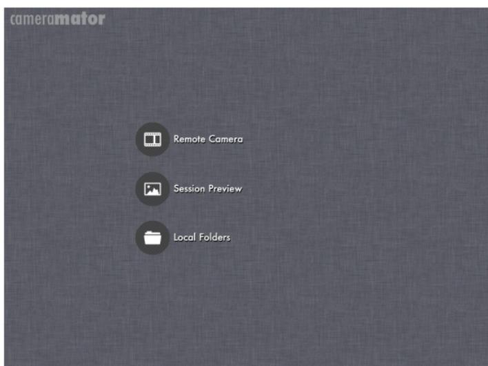
**Remote Camera** – Shows the camera connected to the device. Tapping on the camera name starts the camera control session (see the “Controlling the Camera” section below). Network Settings allow you to change your connection and Wi-Fi preferences.
