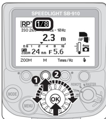
**1** Press function button 2 to highlight the flash output level.
