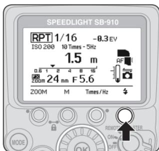
Test fire the Speedlight under the same conditions and with the same Speedlight and camera settings before taking the actual picture.
