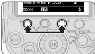
Press function buttons 1 and 3 (a green dot is printed by each button) simultaneously for 2 seconds to reset all settings except custom settings to default.
