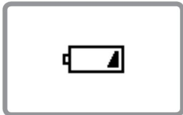
When battery power is low, the icon shown at the left appears on the LCD and the SB-910 stops functioning. Replace or recharge batteries.
