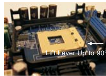
STEP 1: Lift The Socket Lever Up to 90°
