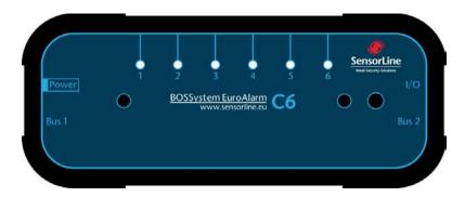
BUS 1/2: Bus connection for system terminals (C6, MP12, SL12)
