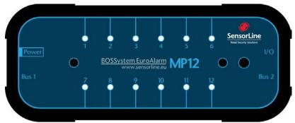
BUS 1/2: Bus connection for system terminals (MP12, SL12, C6) BUS 2: Connect additional terminal or shunt plug if last terminal
