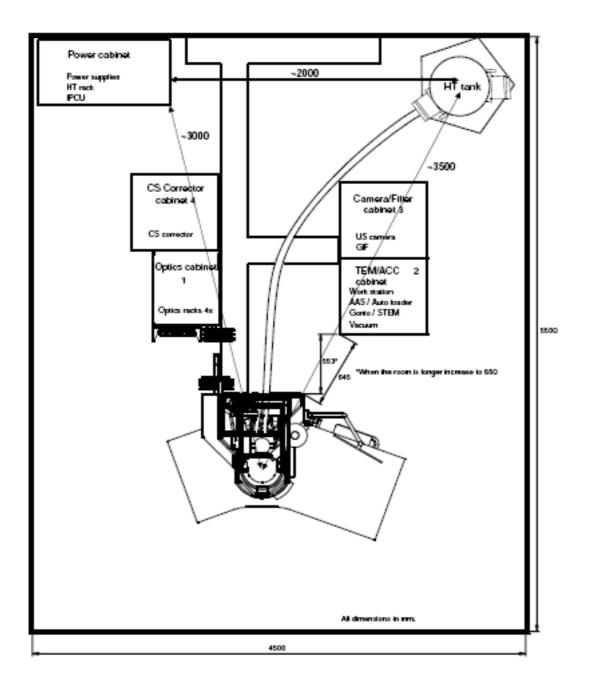
Figure 6: Schematic layout of the electron microscope equipped with a C<sub>s</sub>-corrector.
