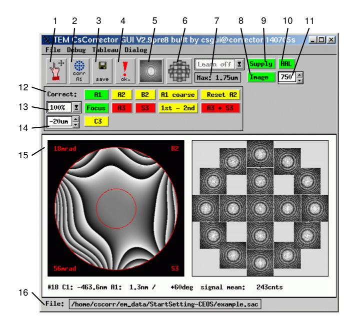
Figure 1: Main window. The auto-alignment tools are displayed. The button No. 1 toggles to the manual alignment tools (see Figure 2), button No. 2 toggles to the auto-alignment tools.
