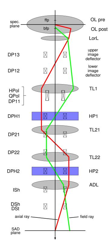
Figure 5: Schematic overview of the electron optical elements of the CETCOR. The corrector is mounted in the column between the objective lens and the projective. The deflectors and stigmators are labeled on the left, round lenses and hexapoles on the right. The image deflector of the microscope is controlled by the CETCOR software using the virtual elements DP12 and DP13.
