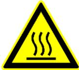
You can burn your skin when touching the inner parts and especially the microplate contact surface and disposables. These parts can reach up to 85°C (185°F)! Do not use materials that are not sufficiently temperature resistant up to 110°C (230°F).
