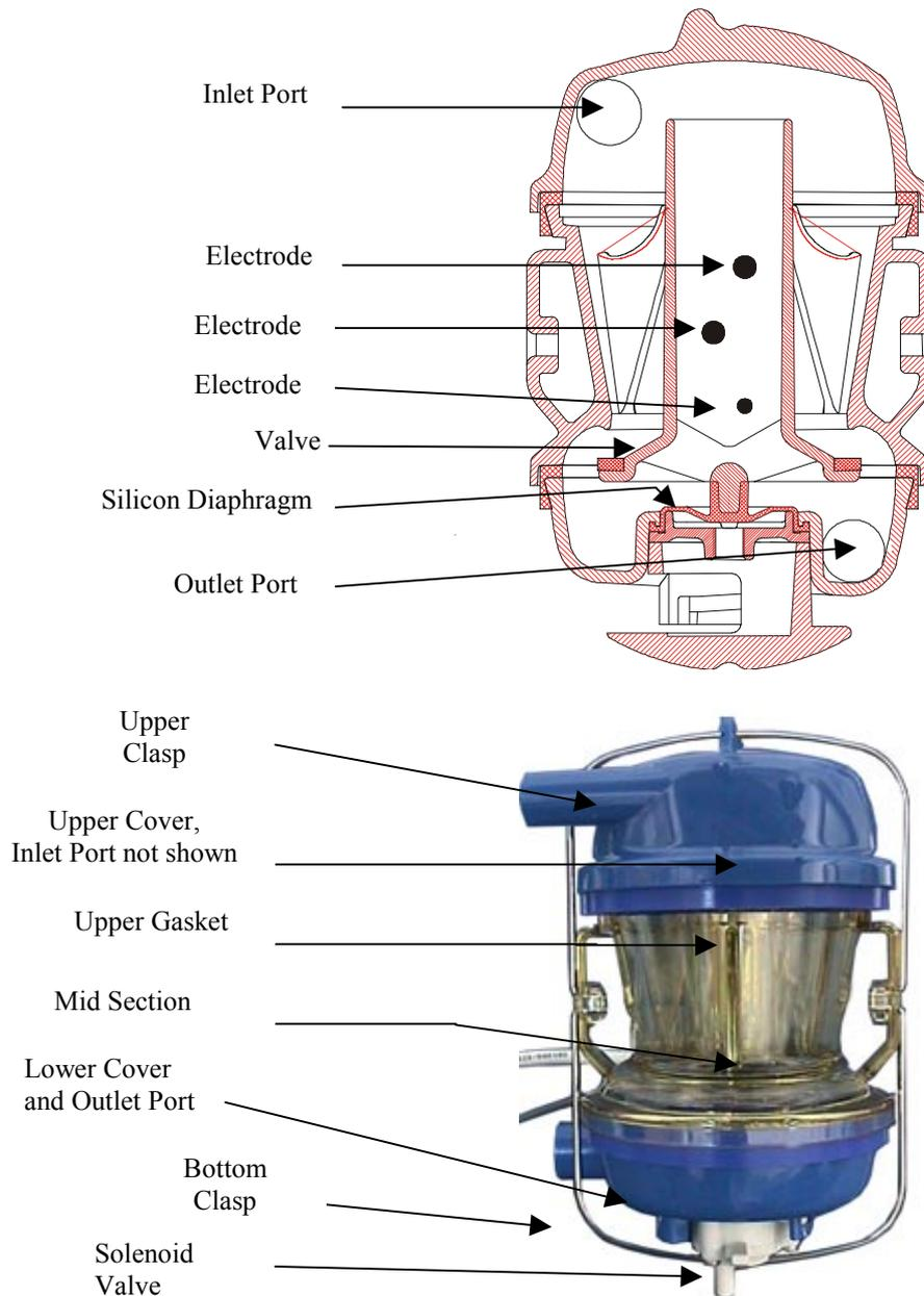
The *AfiFlo* milk meter body is a plastic container made up of three main parts:
