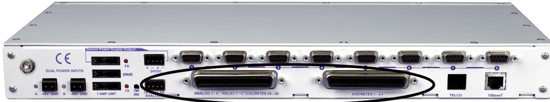
**Fig. 8.** Alarm and control relay connectors
