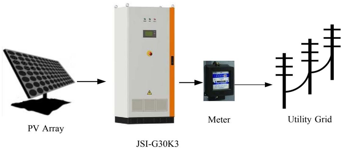
Fig.1 Grid-connected Inverter for PV power application
