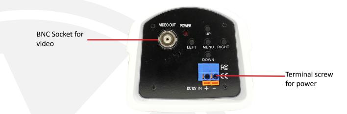
To operate the camera, firstly you will need to connect the BNC and terminal screws to the BNC and DC sockets of a power supply and DVR or Monitor.
