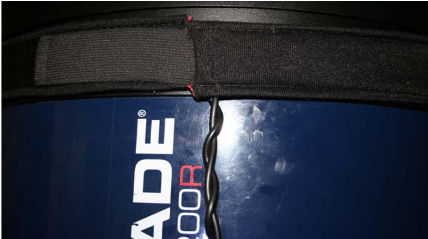
Figure 5 Route Sensor cable with Dew Strap cable
