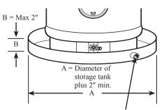
To open drain, this line should be at least 3/4" ID and pitched for proper drainage.
