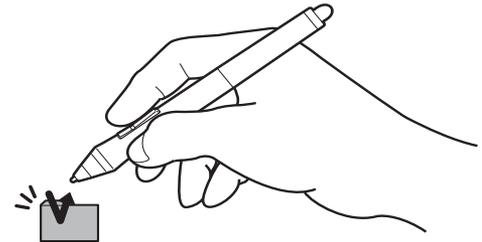
Press the upper side switch (when set to DOUBLE CLICK), or quickly tap the screen twice in the same place with the pen tip. Double-clicking is easier when using the pen perpendicular to the Cintiq's screen.
