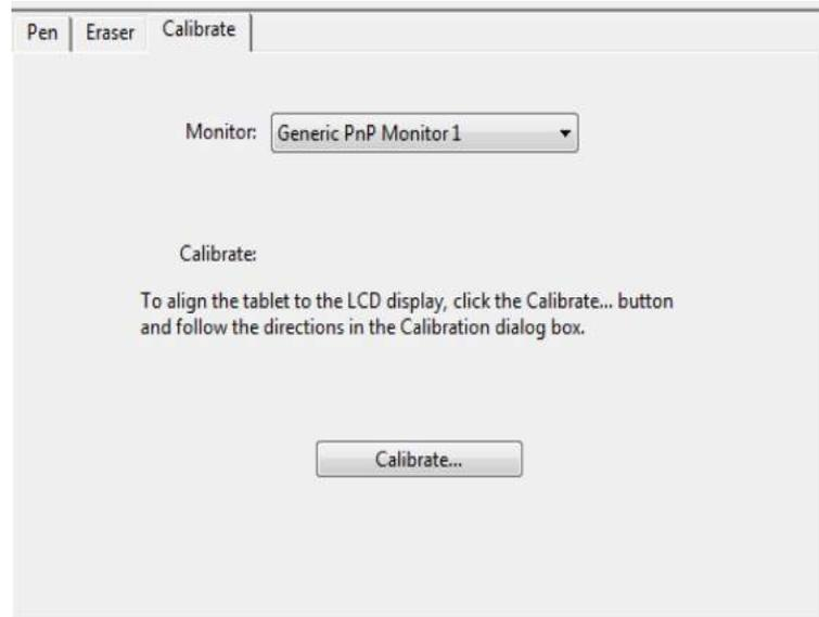
**Tip:** To see the screen cursor slightly offset from the actual position of the pen tip, calibrate by clicking on a spot showing that offset from the crosshairs. For example, to have the screen cursor appear 2.5 mm (1/10th of an inch) above and to the left of the pen tip, calibrate by clicking on a spot 2.5 mm (1/10th of an inch) below and to the right of the crosshairs.
