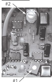
**Trimmer** #1: (see photo) Turning this trimmer CW (clockwise) *increases* the Volume of the pedal only when the pedal is turned ON.
