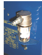
Pneumatic filter, connection to the pneumatic network
