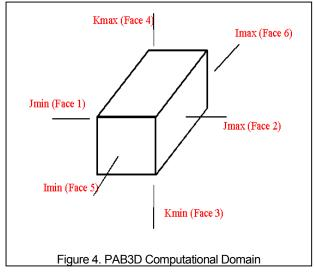
The general multi-block structure in the PAB3D code allows general block connectivity between blocks. Each block can have any dimension, grid topology, and/or the spatial orientation of that dimension. In this case, the entire block can be put in one zone. For each zone (generally, in a multi-block, there is only one zone), there are two lines of input: number of iterations and block dimensions specifications.
