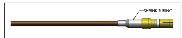
Figure F. Apply shrink tubing.
