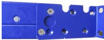
5. Clip the nuts into the holes in the rack you will be using to connect the mounting plates. Check that both sides of the switch are in the same position number on the rack.
