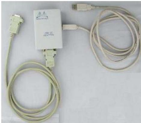
The MTUSB adapter has two connections for cables. One cable is a I2C cable with male connectors on both ends. The other is a USB cable with one type A host connection to be connected to the server or PC and a type B connection to be connected to the MTUSB adapter.
