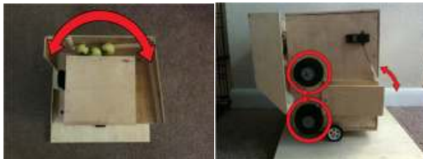
Figure 1: Diagram showing horizontal swivel capability on the machine (Left) and diagram showing launch mechanism along with adjustable launch angle (Right).
