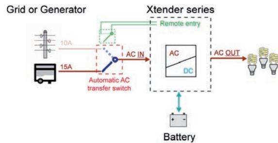
(Figure 5) System on generator connected
