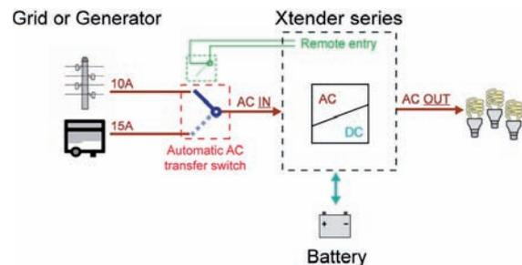
(Figure 6) System simultaneously connected the grid and on a generator
