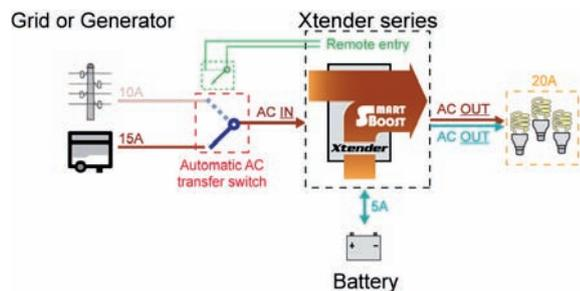
(Figure 7), System with the Smart-Boost function activated
