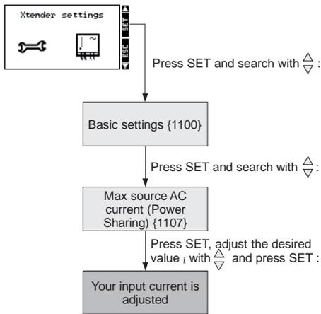
! The current value [Aac] must be set according to the size of the circuit breaker or the grid capacity
