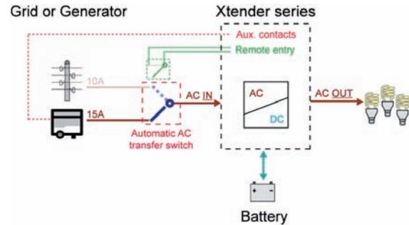
(Figure 8) System with an automatic generator startup
