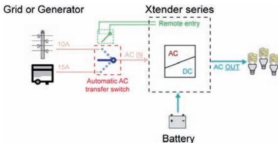
(Figure 4), System in mode "stand-alone"
