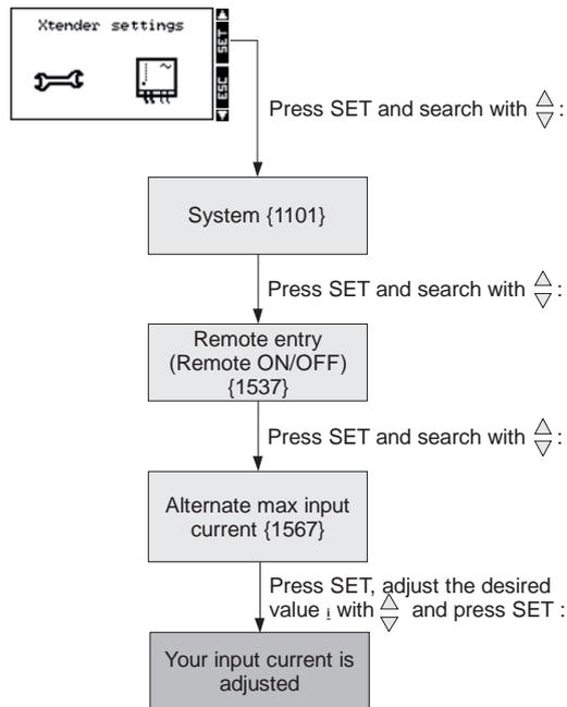
! The current value [Aac] must be set according to the size of the circuit breaker or the grid capacity
