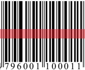
Optimal reading orientation
