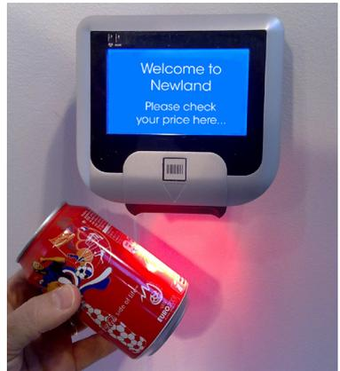
Optimal reading approach to scanner
