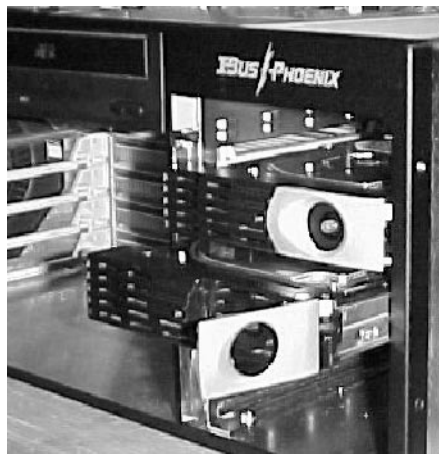
Figure 5-1. Hard Drive Shuttle Partially Withdrawn
