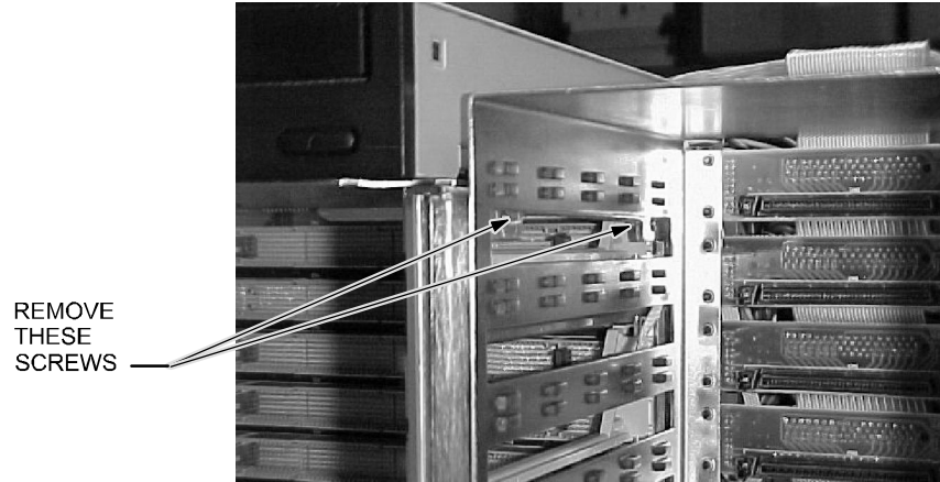
Figure 5-5. Removing the Drive Mounting Plate
