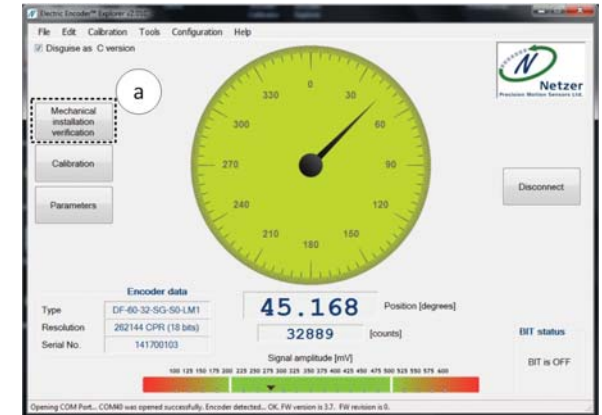
Figure 02: Starting mechanical Installation Verification
