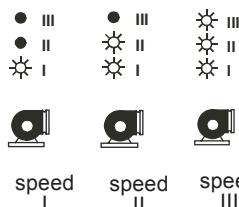
The EAHU operation at a given speed is indicated by the number of LEDs placed at the fan symbol.
