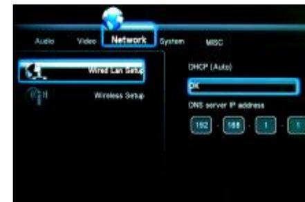
FIX IP (MANUAL) Using Fixed IP, it is required to enter followings. IP address, Subnet Mask, Default Gateway. For further assistant to above settings, please contact to the network administrator. Press ◀ ▶ ▲ ▼ to enter the IP address. Press ENTER to confirm.
