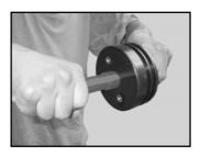
**Step 4 Assemble the Bearing Plate** – Position the bearing plate over the sealing plate, pushing them together so that the threaded portion of the permeate port is visible. Connect the bearing plate and sealing plate with the two interlock screws. A hex wrench can be used to secure the screws.
