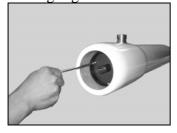
**Step 5 Remove the End Plug** – A male threaded nipple is recommended for use when opening the end plug. Thread the pipe nipple into the permeate port of the end plug, gently motion the nipple in various directions, and then gently pull the nipple from the vessel. A firm tug may be required to release the end plug o-ring seal.
