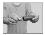
**Step 6 Install Adapter** – The adapter should be pushed into the permeate port until the wider diameter middle section is flush against the end of the permeate port. Simultaneously pushing and turning the adapter will ease installation.
