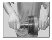
**Step 7 Install Head O-ring -** All o-rings should be coated with a thin layer of glycerine before installation. Seat the head o-ring into the groove on the outside diameter of the head.
