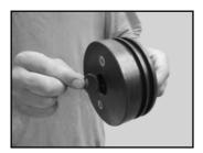
**Step 3 Assemble Permeate Port** – Install the permeate port into the sealing plate.
