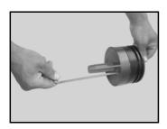
**Step 5 Install Adapter O-rings** –All o-rings should be coated with a thin layer of glycerine before installation. Care should be used to minimize the amount or glycerine applied and any excess should be removed. Seat one o-ring into each of the two grooves located at the element end, inside diameter of the adapter.
