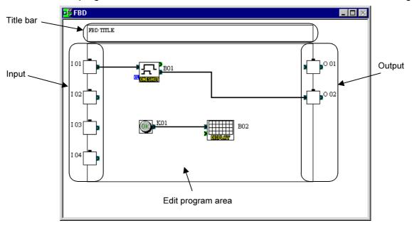
The user can perform the following ten operations using FBD window. Refer to Chapter 6 for more details. The size for edit program area can be changed by the operation of mouse.
