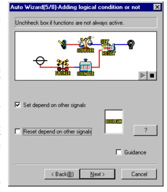
When adding check this option, the input signal can be connected to left most Set/Reset function block connected to the reset pin side of the Flicker or Compere function block.
