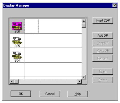
4) Click the "Add DP" button to add DP function block(s) for the CDP function block. It is possible to add a maximum of 10 DPs into 1 CDP.
