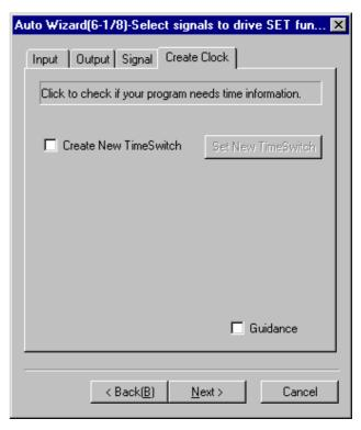
b) Click the "Set New TimeSwitch" button to set parameter for the Time Switch function block. A setting operation is identical to the parameter of the Time Switch function block set on the FBD base. Further information about parameters of each function block can be found in the programming manual and "Help" on the AL-PCS/WIN-E.
