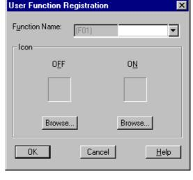
b) Choose the ON or OFF image from the Open window. Then, click the "Open" button to register the ON or OFF image.
