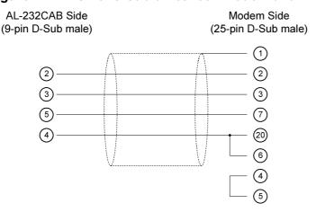
11.2.2 RS-232C Straight Cable Between Modem (GSM Modem) and AL2-GSM-CAB (Model Type: AL2-14M\*-\*, AL2-24M\*-\*)
