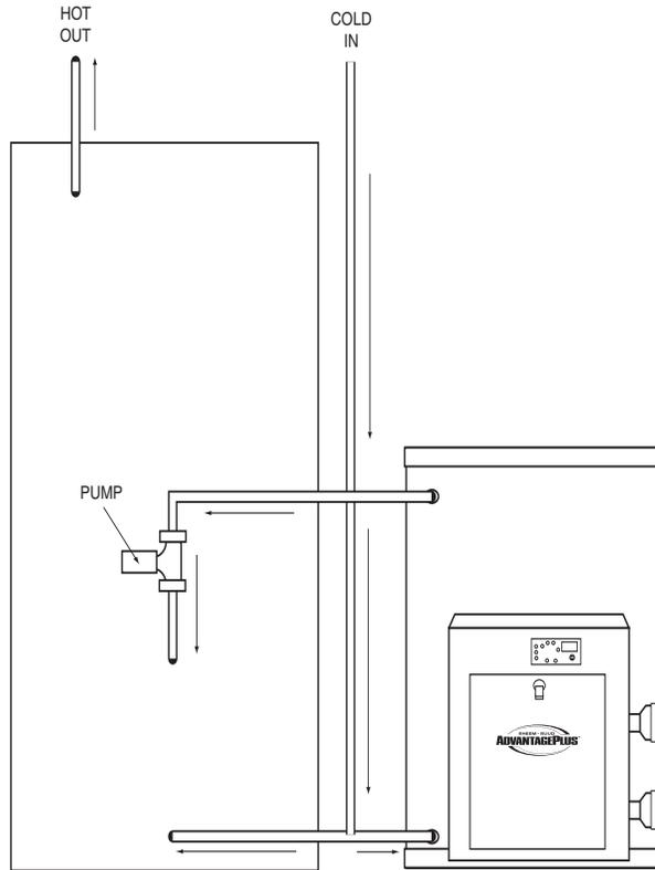
**Sample Reverse Manifold and Piping Diagram for the AdvantagePlus.
