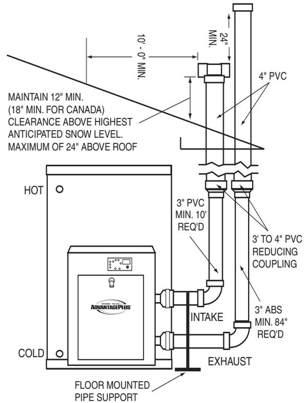
FIGURE 6 - VERTICAL ROOF VENTING
