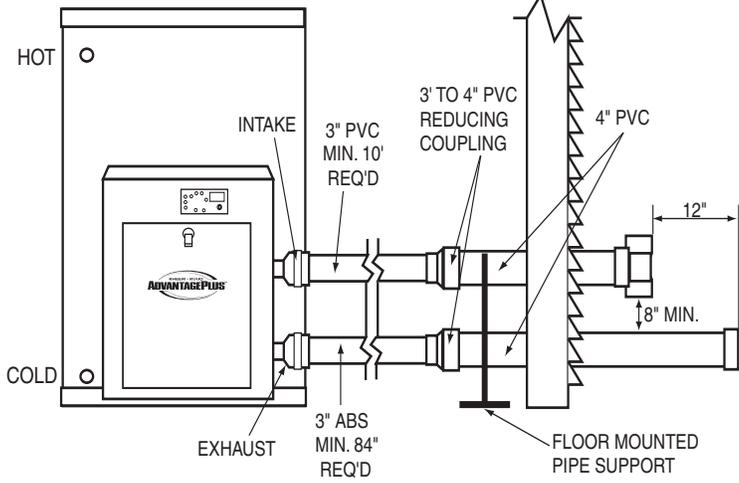
FIGURE 5 - SIDE WALL VENTING
