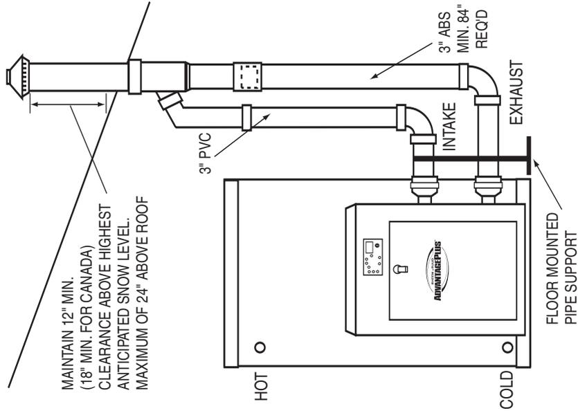
FIGURE 3 - VERTICAL ROOF VENTING
