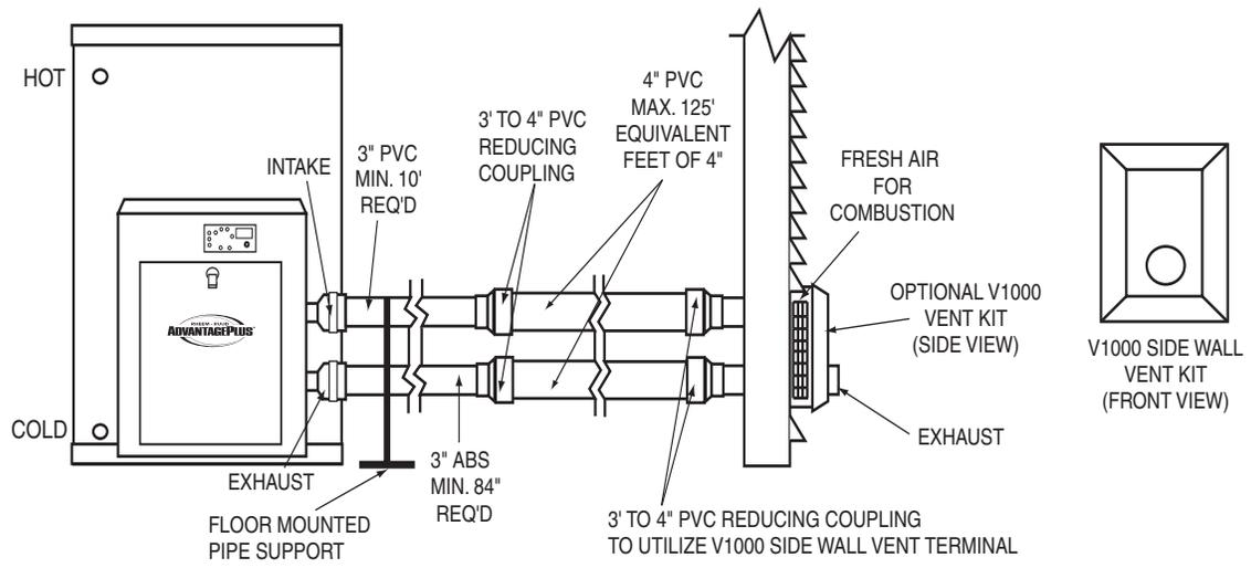
FIGURE 7 - SIDE WALL VENTING USING THE V1000 VENT KIT
