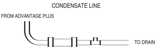
CONDENSATE LINE MUST BE PITCHED AT LEAST 1/4" PER FOOT TO PROPERLY DRAIN. IF THIS CANNOT BE DONE OR A VERY LONG LENGTH OF CONDENSATE HOSE IS USED YOU MUST INCREASE THE CONDENSATE HOSE TO A MINIMUM OF 1" I.D. AND PLACE A TEE IN THE LINE AFTER THE CONDENSATE NEUTRALIZER TO PROPERLY REDUCE VACUUM LOCK IN THE DRAIN LINE.
