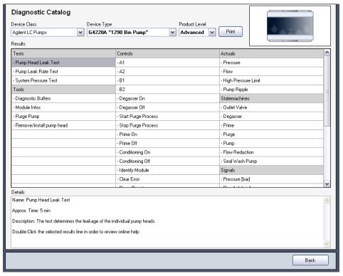
The Diagnostic Catalog is a catalog of all tests, calibrations, tools, instrument controls and EMF counters for each module at each Lab Advisor product level. The list is filtered by **Device Class** (that is, instrument or module type), **Device**
