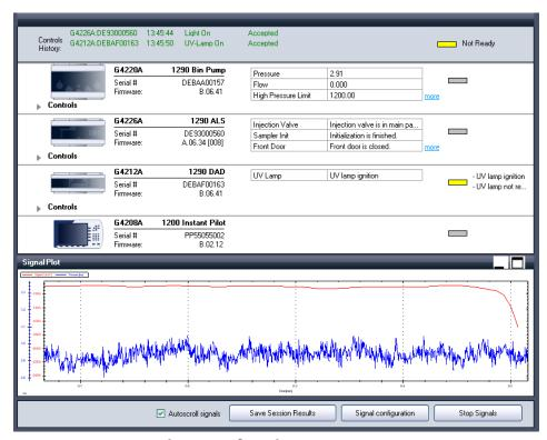
The Reply Panel of the **Instrument Control** screen displays any replies generated from the device, to verify that the control used was accepted; it shows only the last three replies. In order to get a complete history of replies, click **Save Session Results** in the Action Panel. The reply history is saved and can be viewed in the **Logs & Results** screen.
