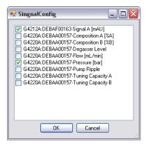
The selected signals are visible in the Signal Plot starting in "lanes" mode, which divides the available area of the window between the number of configured signals. This gives each signal a limited size in the window, but all are easy to differentiate and each scale is shown on the left side of the plot.
