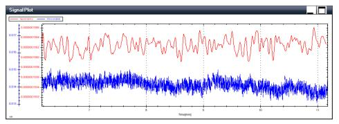
Other scaling parameters can be selected by right-clicking the signal window and selecting the **Auto Scaling** from the context menu. The available scaling options are presented in the submenu.
