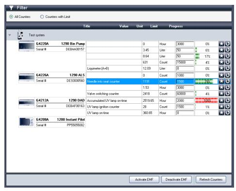
The EMF screen can be used to view all possible counters or, for better overview, to filer only those counters that have an activated limit.
