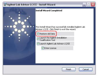
If B.01.xx is uninstalled after the installation of the B.02.xx, then the restore can be activated by navigating to the application folder, typically ..\Program Files\Agilent Technologies\Lab Advisor and double-clicking the Agilent.InstrDiag.DataMigration.exe program.
