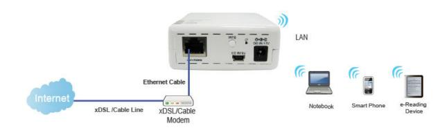
The WAN access type is depended on the service that you contract with the provider. The 802.11n HSPA Mobile Router provides five selections for the WAN access type, **Static IP**, **DHCP Client, PPPoE, PPTP, L2TP**. Check with your ISP if you don't know the WAN type.
