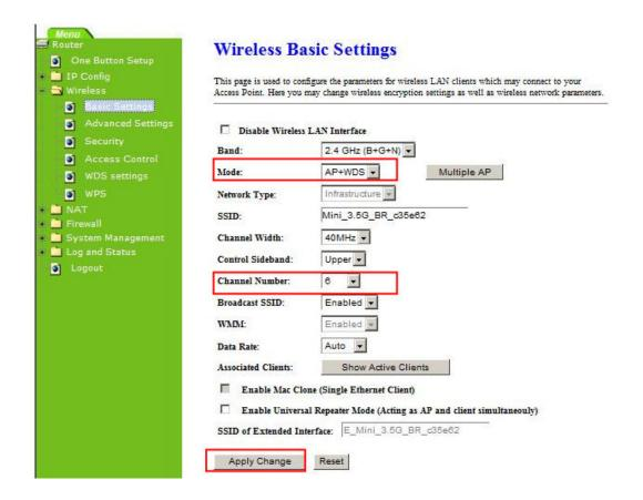
(3) Enable WDS function from the page – "WDS Setting", and then fill in the MAC address of Router B. Click Apply Changes to save the setting data.
