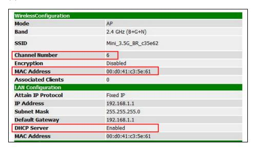
(2) Set the connection mode to "AP+WDS" from "Wireless Basic Setting", and then select the channel number (in this example is "6"). Click Apply Changes to save the setting.
