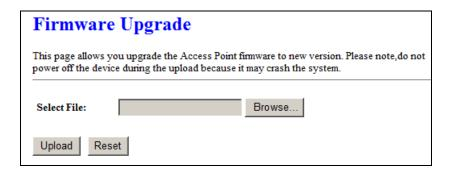
Note: 1. To prevent that firmware upgrading is interrupted by other wireless signals and causes failure. We recommend users to use wired connection during upgrading.
