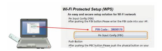
(2) Fill in the PIN number from the wireless card in Client PIN Number field, and then click "Start PIN".
