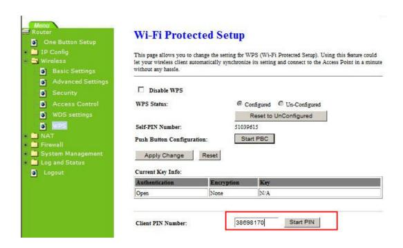
(3) Click PIN from Adapter Utility to complete the WPS process with the wireless router.
