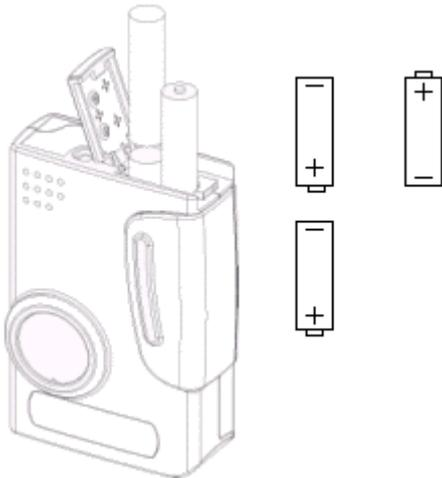
**Figure 2: inserting batteries**
