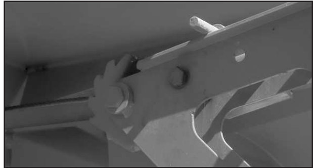
Figure 11 – Cradle fastened by locking lever.
