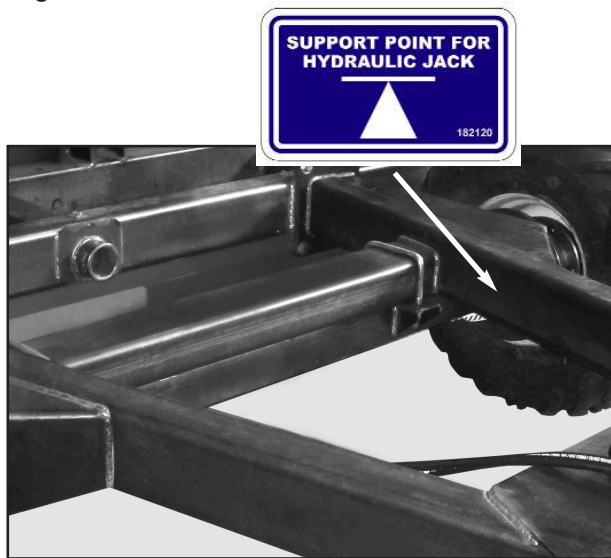
Figure 2 - Support point for jack location
