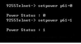
setpower p61=1: Port On setpower p61=0: Port Off
