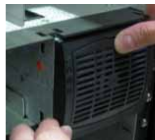
Fig. 3.10 Unlocking and locking an inverter module for removal or insertion
