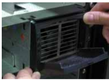
Fig. 3.10 Unlocking and locking an inverter module for removal or insertion
