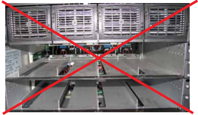
Unsafe solution. Do not leave any module slots open.
