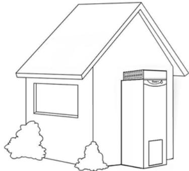
The water heater must not be installed in an area with a corrosive atmosphere where chemicals are stored or where aerosol propellants are released. Remember the air may be safe to breathe, but when it goes through a flame, chemical changes take place which may attack the water heater.
