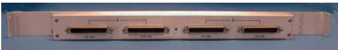
Breakout panel (front). Use RJ-21 high-density cables to connect to transition card
