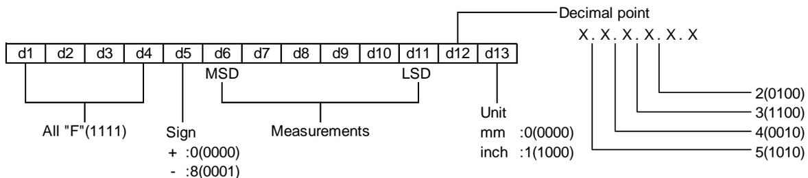
※This instrument outputs 13 digits from d1 to d13 by making 4 bits into 1 digit.
