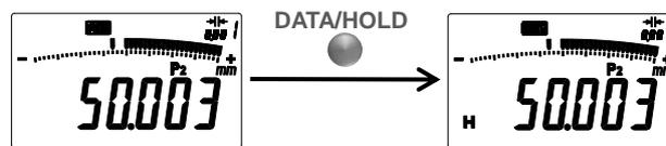
(Note) Hold the display value is performed at the same time when the data processor is not connected.
