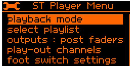
Use the Up/Down buttons, to navigate to the desired menu setting. Use the Select button to choose the settings. Use Up/Down to modify values and Select to confirm the changes. Back button can be used to go one level back without changing the parameters.
