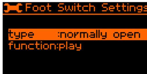
Type: Adjust the “type” setting to tell the LP-16 if you are using a “normally open” or “normally closed” type footswitch. Consult your footswitch’s documentation to determine which type you have.
