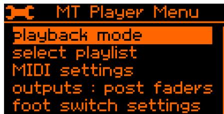
Use the Up/Down buttons, to navigate to the desired menu setting. Use the Select button to choose the settings. Use Up/Down to modify values and Select to confirm the changes. Back button can be used to go one level back without changing the parameters.
