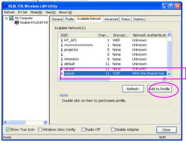
If the wireless access point uses encryption, you have to input WEP passphrase or WPA preshared key. Please ask the owner of the wireless access point you want to connect, and input the correct passphrase / preshared key at "Network key" & "Confirm network key", then click 'OK'.
