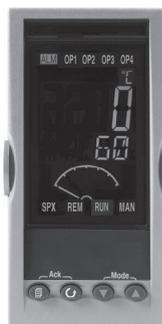
Measured Temperature or Pressure (Process Value 'PV')
