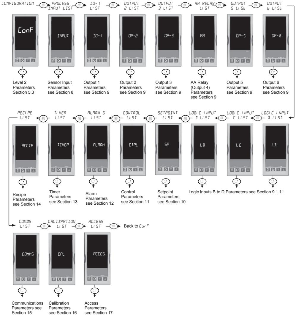
In SX80 controllers some lists are not available, for example Output 5, Output 6, and Digital Communications. In SX80 Logic Inputs A and B are available, Logic Inputs C and D are not available.
