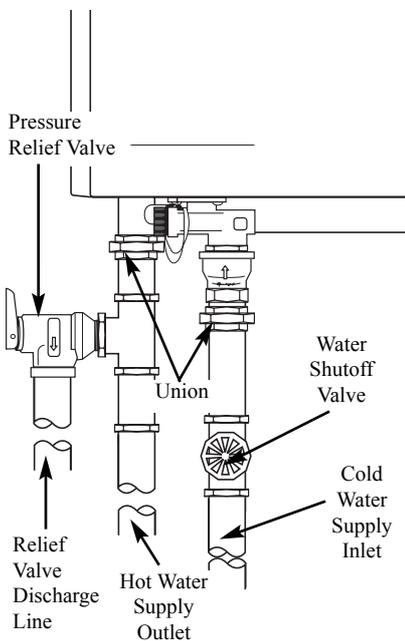
**Notice:** The above illustrates a pressure only relief valve. If local codes require a combination temperature and pressure relief valve be installed, an extension piece may be needed. (Refer to page 16 for example of extension piece for T&P relief valve installation.)
