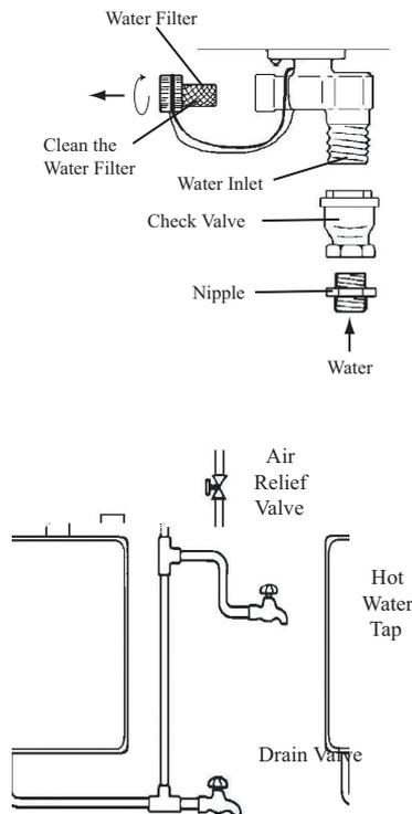
Install a shutoff valve near the inlet of the water heater for service and draining purposes.
