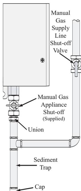
It is recommended that a Manual Gas Appliance Shutoff Valve be installed at the gas connection of the water heater at the time of installation (see diagram to the left).
