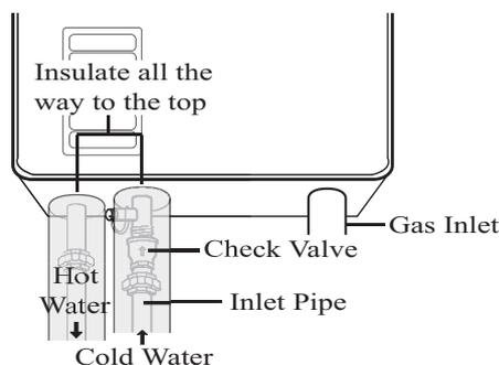
For increased energy efficiency, use pipe insulation. Please install the insulation, according to the illustrations above,
